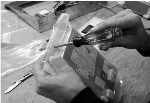
6. While holding down the folded poly-vinyl, insert a screwdriver, punch, or knife point thru the folded plastic and the mounting hole until it protrudes through the bag on the opposite side. Repeat this step to punch a hole in the other mounting hole.
