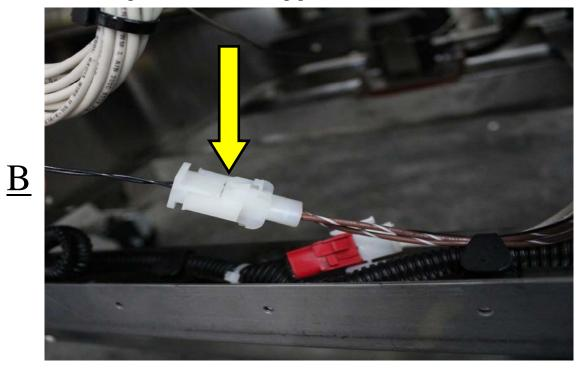
10. Insert short cable 2 pos connectors between existing probe connectors (see illustration-C)
