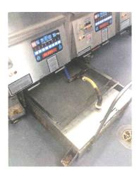
Gycor Filter Powder Pads need to be placed in a completely dry filter machine. We recommend that the filter machine be cleaned out the night before and the parts allowed to air dry overnight. A new filter pad should be installed prior to filtering, but not the night before.
