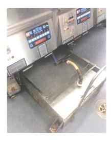
• Push filter pan back into place and make sure that it is completely in. Connect pump hose and return hose before filtering.
